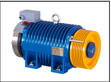
Gearless Machine A gearless elevator machine is a type of traction machine used in modern elevator systems. Unlike traditional geared traction machines, which employ a gearbox to increase torque, gearless machines directly couple the motor to the traction sheave.
