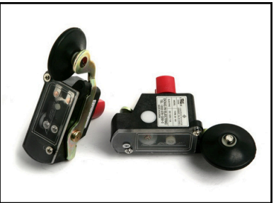
Limit Switch Elevator limit switches are safety devices that play a crucial role in the safe operation of elevator systems. They are designed to detect the position of the elevator car within the hoistway and signal the elevator control system to stop or change direction when certain predetermined limits are reached.
